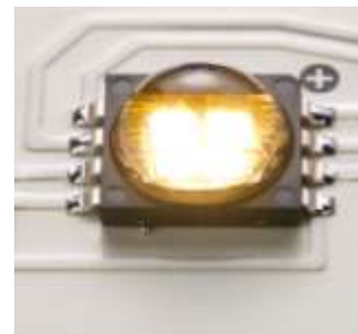
Elliptical Optic 10395 "Note the dark line caused by the gap in the chips"
